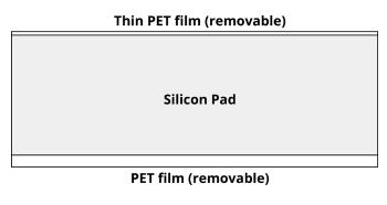
A full silicone pad covered with a PET film on both contact surfaces for increased stability and easy installation. Both are to be removed for installation.
